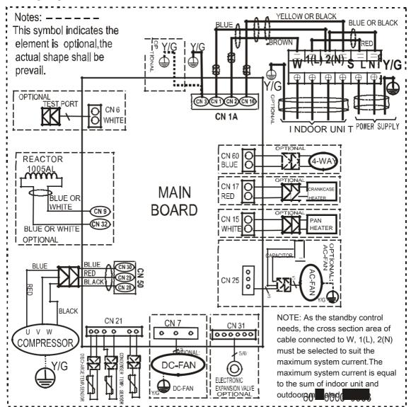
Outdoor unit wiring diagram: 16022000019069
