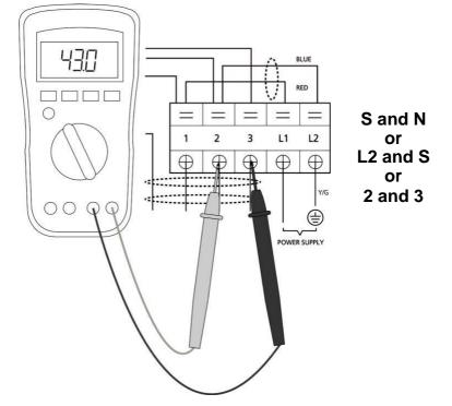
Use a multimeter to test the resistance of the reactor which does not connect with capacitor. The normal value should be around zero ohm. Otherwise, the reactor must have malfunction.
