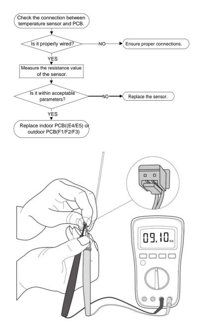
Note: For certain models, outdoor PCB could not be removed separately. In this case, the outdoor electric control box should be replaced as a whole. This picture and the value are only for reference, actual appearance and value may vary
