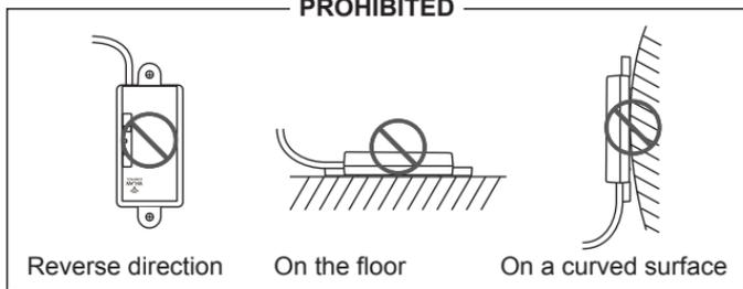
Do not lay the WLAN adapter cable on the floor. You may trip on the cables.
