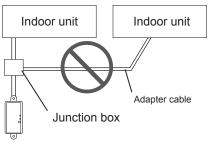
(4) Extended wiring Extending the cable is prohibited.
