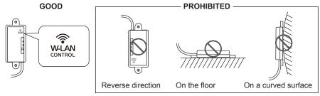
Do not lay the WLAN adapter cable on the floor. You may trip on the cables.
