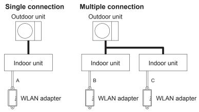
A, B, and C: Adapter cable attached to this product.
