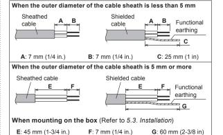
When the cable is along the wall (Refer to 5.3. Installation)
