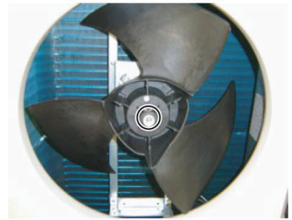
Remove the Hex Socket Screw. And remove the PROPELLER FAN. Note at the installation. Insert propeller Fan and Moter shaft reference D cutting position. And the tightening torque at the installation. Tightening torque is from 10 to 15N.M.
