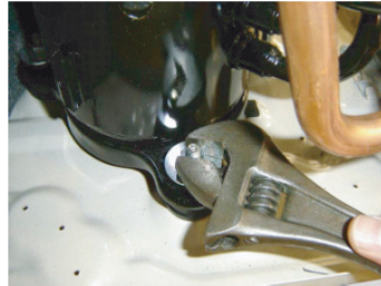
Remove the COMP BOLTS. (3 place)
