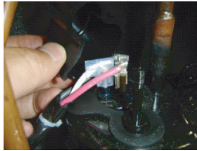
Remove the connectors. [R : RED, C(T) : BLACK, S(W) : WHITE]
