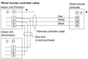
\*Earth (Ground) the remote controller if it has a earth (ground) line.
