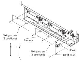
Install the barriers in the correct direction.
