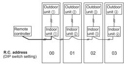
: Transmission cable, Power supply cable : Power supply cable Remote controller cable -//- · Bus wire
