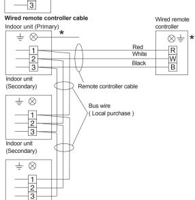
\*Earth (Ground) the remote controller if it has a earth (ground) line.
