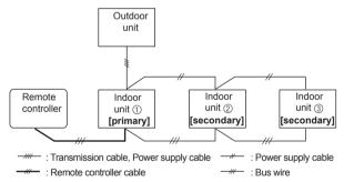
(2) Set the R.C. address (DIP switch setting)
