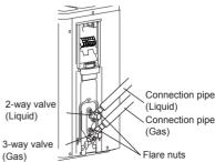
(4) When the flare nut is tightened properly by your hand, use a torque wrench to finally tighten it.
