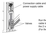
Run the connection cable and power supply cable to the rear of the outdoor unit between the 2 valves as shown in the figure (For the switch cover to be easily installed.)
