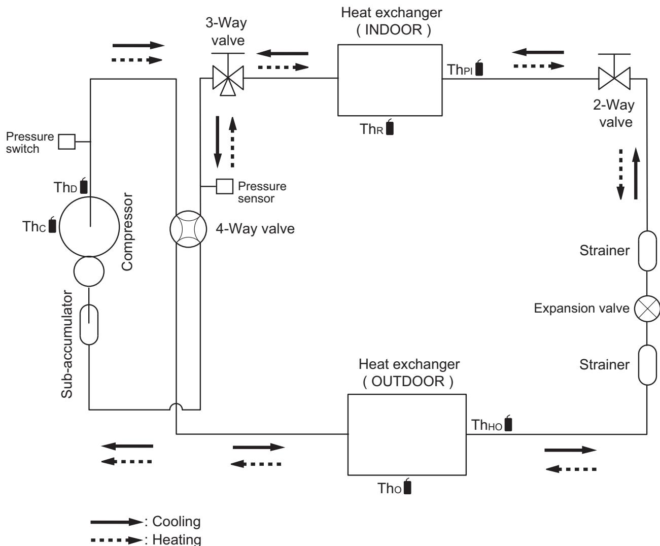
Thc : Thermistor (Compressor temperature)
