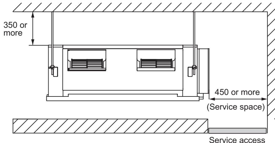
Installation by which service space is carried out from the bottom of the unit.
