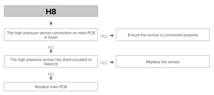
1 Measure the resistance among the three terminals of the pressure sensor. If the resistance is of the order of mega Ohms or infinite, the pressure sensor has failed.
