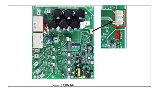
Situation 1: L1 or L2 error is displayed immediately after the outdoor unit is switched on
