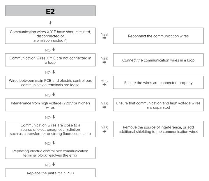
1 Measure resistance between X Y E. Normal resistance between X and Y is 120Ω. Communication wiring has polarity. Ensure wire X is connected to terminal X, etc.
