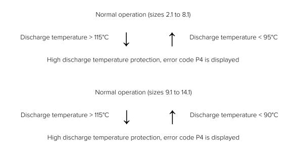
When the discharge temperature rises above 115°C, the system displays P4 protection and the unit shuts down. When the discharge temperature drops below 95°C, the compressor enters re-start control.
