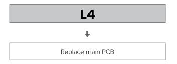
Situation 2: L4 error is displayed after the compressor has been in operation for a period of time and the compressor speed is over 60 rps
