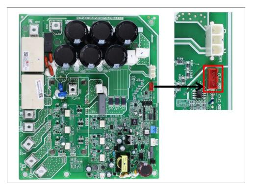
When replacing an inverter module, a layer of thermally conductive silica gel should be painted on the IPM module (on the reverse side of the inverter module PCB).
