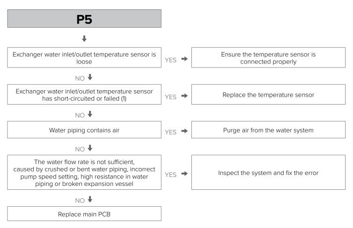
1 Measure sensor resistance. If the resistance is too low, the sensor has short-circuited. If the resistance is not consistent with the sensor's resistance characteristics table, the sensor has failed.
