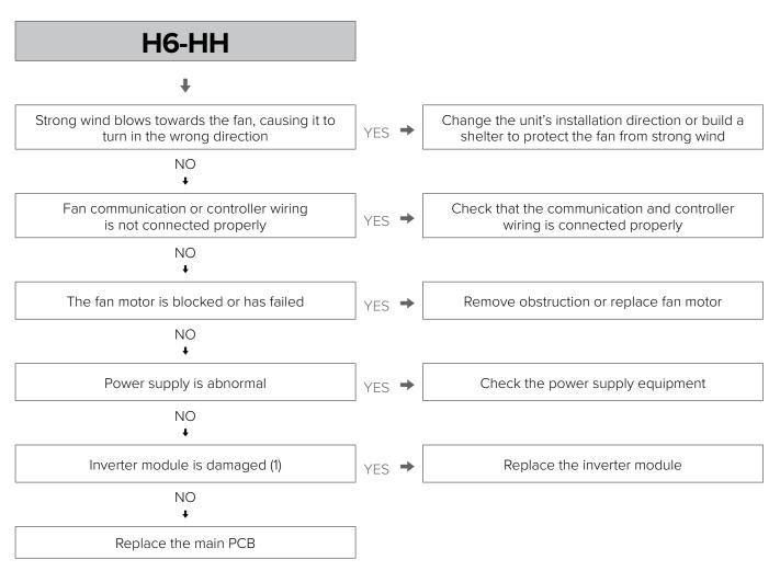
1 Measure the voltage between the black and white wires of the DC fan motor power output. The normal voltage is 15V when the unit is in standby. If the voltage is significantly different from 15V, the IPM module on the inverter module is damaged.
