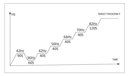
4.3.2.3 Sizes 2.1 - 3.1: ambient temperature at or lower than 3°C Sizes 4.1 - 5.1: ambient temperature at or lower than 11°C
