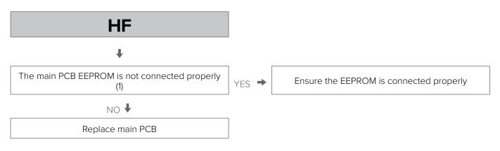
1 The unit EEPROM is assigned IC320 on single-phase unit WiSAN-YME 1 S 2.1 - 5.1, assigned IC14 on singlephase unit WiSAN-YME 1 S 6.1-8.1 and assigned IC25 on unit WiSAN-YME 1 S 6.1T-14.1
