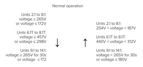
Compressor voltage protection, error code H7 is displayed
