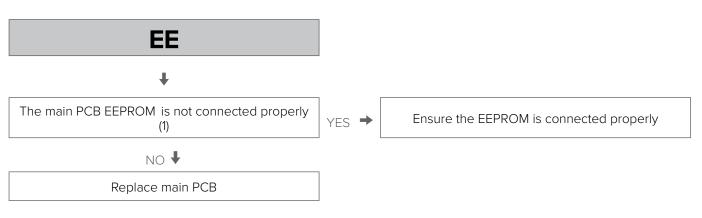
1 Hydronic system main PCB EEPROM is assigned on hydronic system main PCB.
