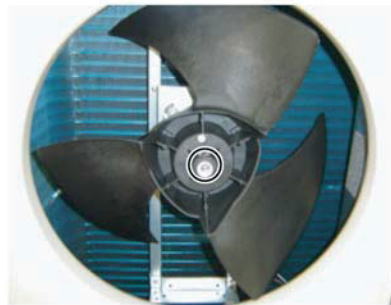
Remove the Hex Socket Screw. And remove the PROPELLER FAN. Note at the installation. Insert propeller Fan and Moter shalf reference D cutting position. And the tightening torque at the installation. Tightening torque is from 10 to 15 N.M.
