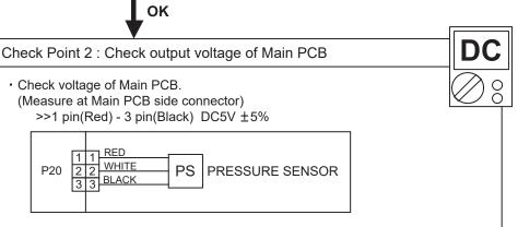
▶ If the voltage is not correct, replace Main PCB.
