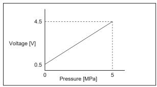
▶ If the voltage is not correct, replace Presure Sensor.
