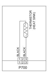
► If the voltage does not appear, replace Inverter PCB, and execute the check operation again.
