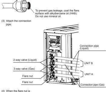
tightened properly by your hand, use a torque wrench to finally tighten it. Body side 90° Torque wrench
