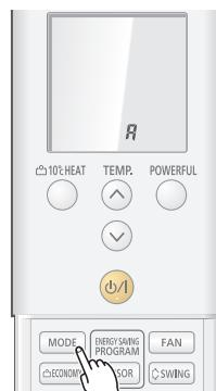
3. Press the TEMP. " ^ " or the " v " button to change the custom code between A → b → c → d.
