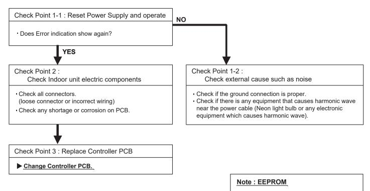
EEPROM(Electronically Erasable and Programmable Read Only Memory) is a nonvolatile memory which keeps memorized information even if power is turned off. It can change the contents electronically. To change the contents, it uses higher voltage than normal, and it can not change a partial contents. (Rewriting shall be done upon erasing the all contents.) There is a limit in a number of rewriting.
