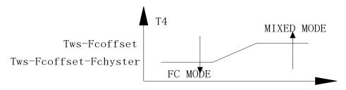
When T4<Tws-Fcoffset-Fchy, unit switch in FC MODE
